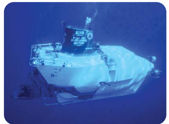
Figure 6 The Alvin carries one pilot and two scientists. It has underwater cameras, lights, a television system, and instruments to collect samples from the water.
